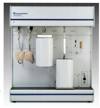
Micromeritics introduces the new ASAP 2020 HD which includes many features that offer improved isotherm resolution and accuracy. Current ASAP 2020 users can also benefit from these new capabilities by upgrading their instrument to the new HD standard.
