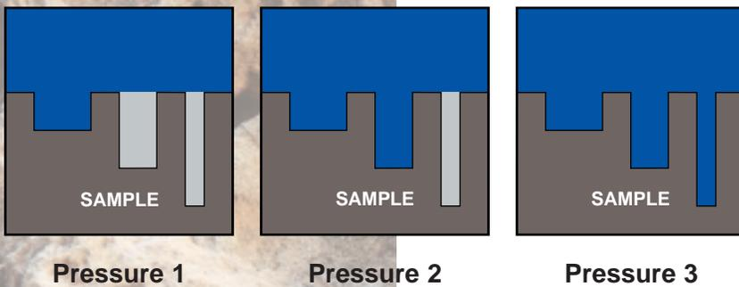
As pressure on the filled penetrometer increases, mercury intrudes into the sample's pores, beginning with those pores of largest diameter. This requires that mercury move from the capillary stem into the cup, resulting in a decreased capacitance between the now-shorter mercury column inside the stem and the metal cladding on the outer surface of the stem.
