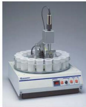
The MasterTech features a powerful ultrasonic probe for sample redispersion. Power to the probe tip is adjustable and the driving
