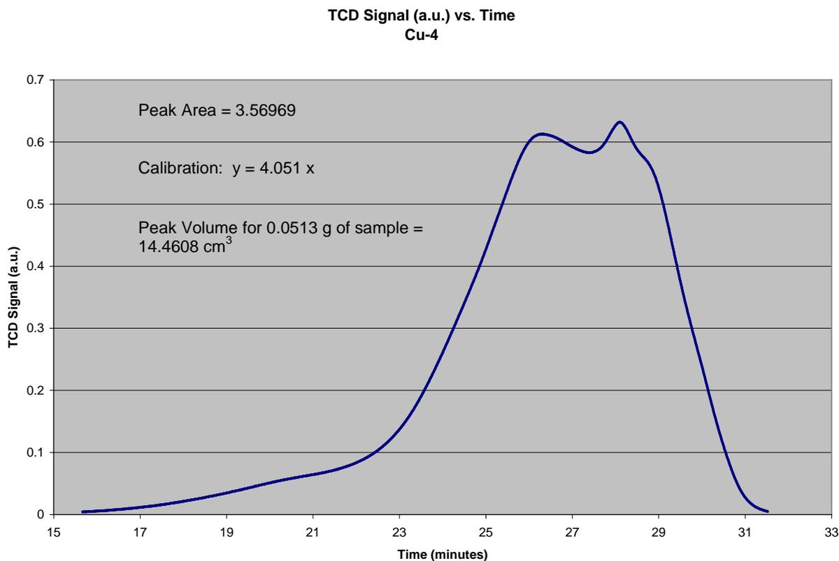
The sample file used a CuO weight of 0.0513 grams and consumed  $14.46 \text{ cm}^3$  of hydrogen gas or  $281.89 \text{ cm}^3$  hydrogen gas per gram of copper oxide. Again, the theoretical amount of hydrogen gas for this reduction is  $281.78 \text{ cm}^3$  so the experimental hydrogen consumption was 100.04% of theoretical.
