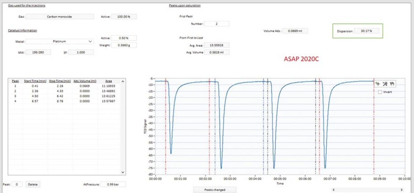
Figure 4: Pulse chemisorption results for a reference Pt/alumina reference catalyst, measured by connecting the ICCS to an ASAP 2020C, are consistent with previous results and published data for the material.
