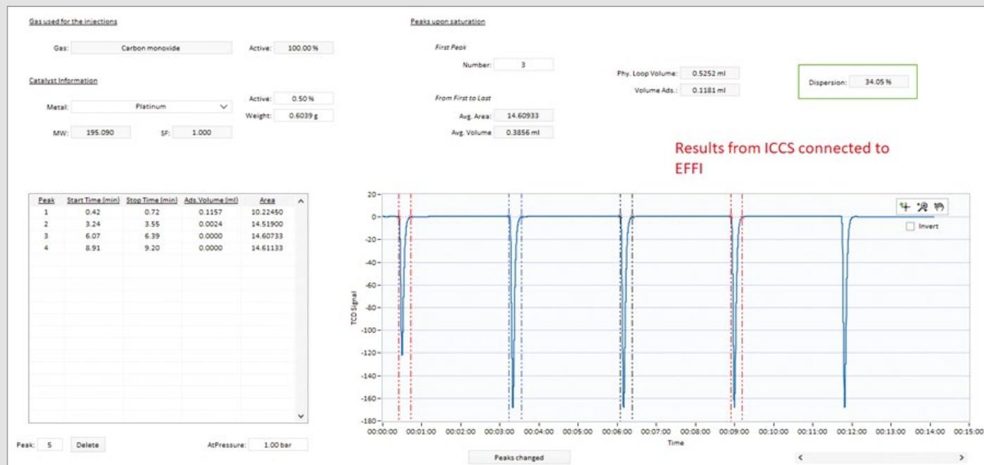
Figure 2: Pulse chemisorption results for a reference Pt/alumina reference catalyst, measured by connecting the ICCS to a Microactivity Effi, are consistent with published data for the material.
