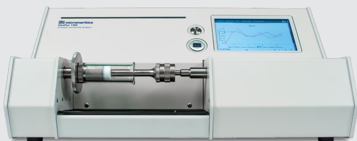
The GeoPyc measures envelope volume by solid phase displacement
