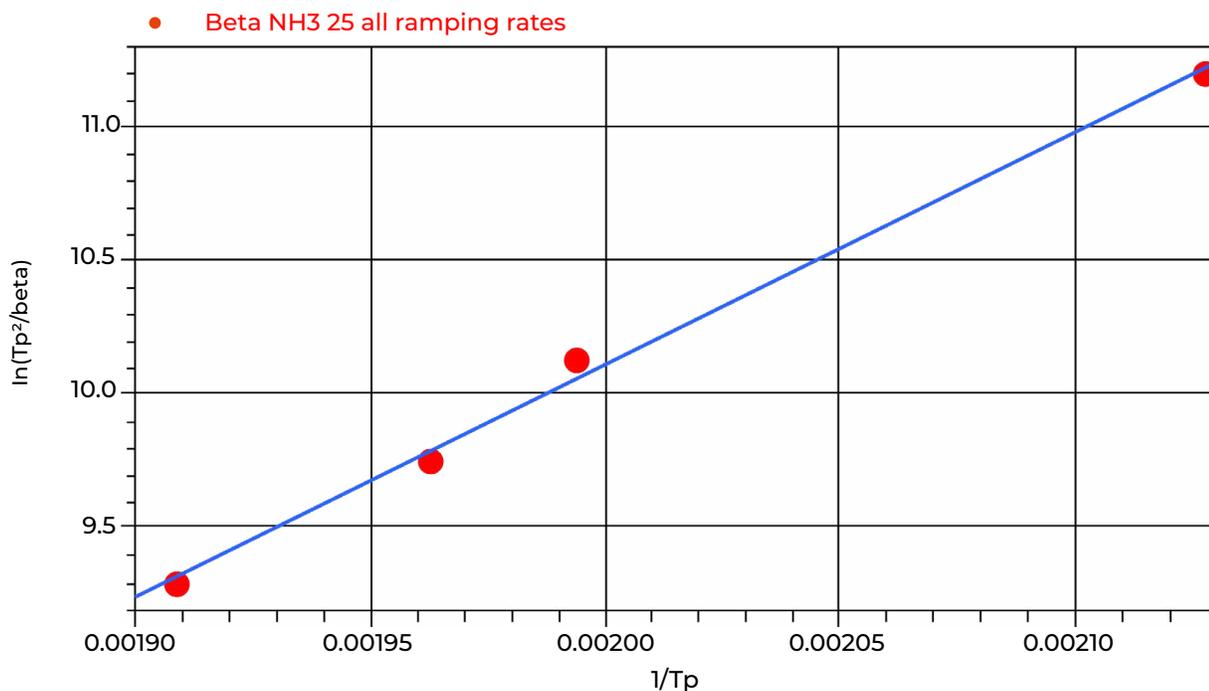
**Figure 4.** First order desorption kinetics plotted from consecutive TPD experiments on beta zeolite. One sample prep was used for four TPD's.
