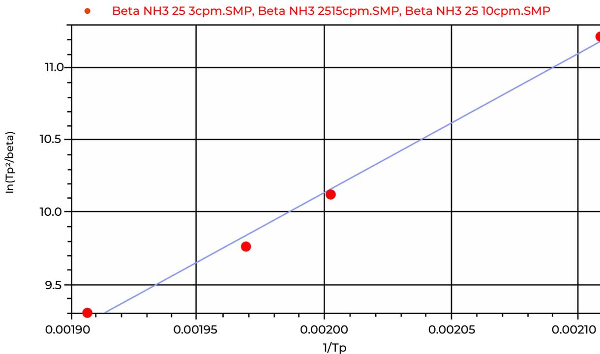
**Figure 5.** First order desorption kinetics plotted from separate TPD experiments with different ramp rates on beta zeolite. A fresh batch of beta zeolite was prepared for each TPD experiment.
