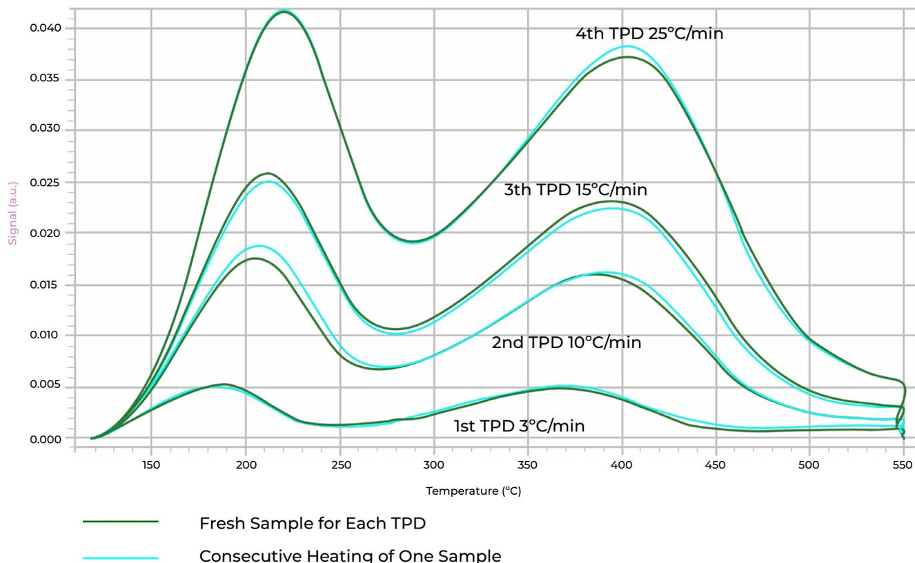
**Figure 3.** Ammonia TPD of ZSM-5 with separate and consecutive temperature ramps.
