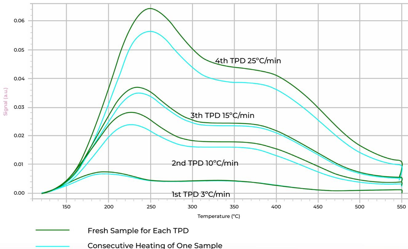
**Figure 2.** Ammonia TPD of beta zeolite with separate and consecutive temperature ramps.
