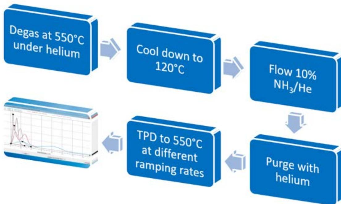
**Figure 1.** An example of ammonia Temperature Programmed Desorption (TPD) experiment.
