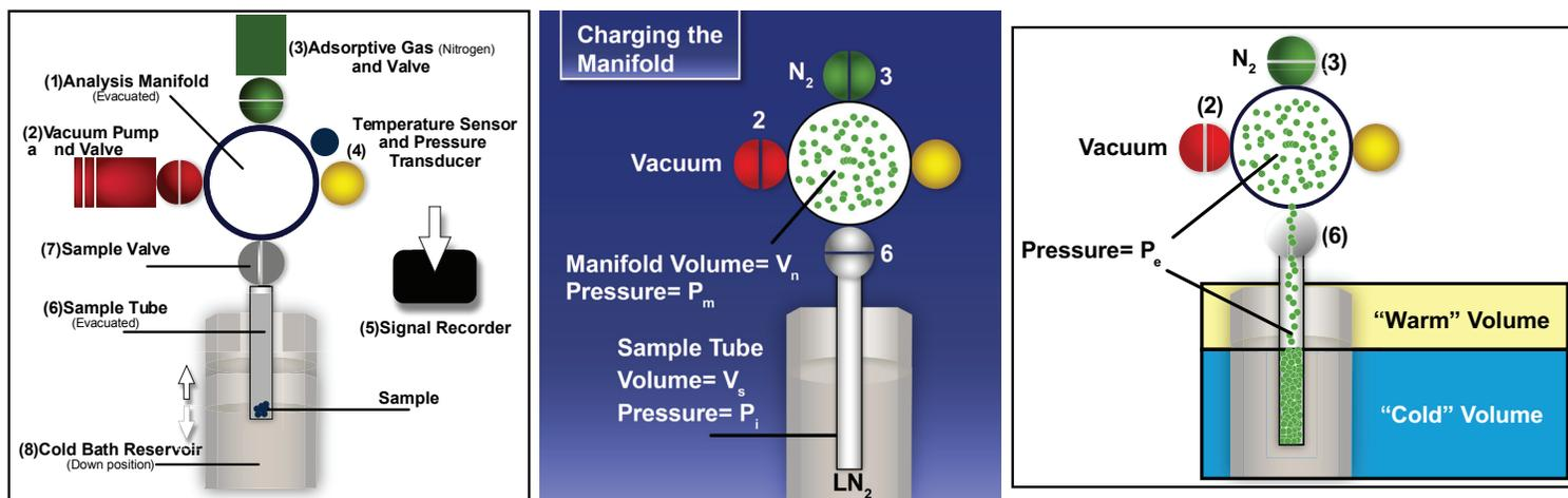
Figure 1: A simple schematic of a generic, volumetric gas adsorption analyzer showing, from left to right – degassing, charging of the manifold, and gas adsorption onto the sample.
