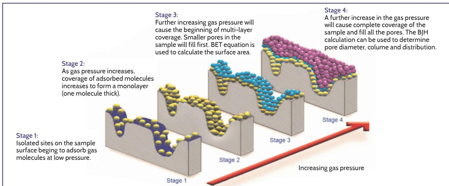
Figure 2: In a gas adsorption measurement the pores of the sample progressively fill with the adsorptive gas as pressure is increased.
