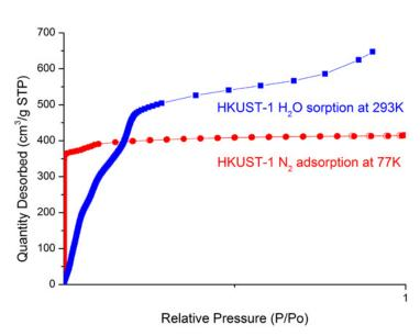
Figure 1. Nitrogen sorption isotherm of HKUST-1 (Red), water vapor sorption isotherm of HKUST-1 (Blue)
