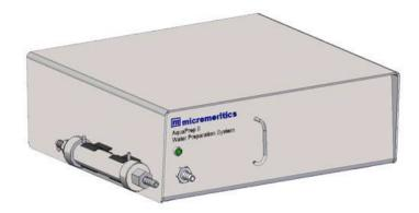
The air removed from the water is exhausted through a small tube also at the front of the instrument. Placing a small beaker of water around the tube so that its vent is submerged reveals by its bubbling the rate of air removal. This guides you in assessing when sufficient air has been extracted from the water. Not all dissolved air has to be removed for satisfactory use with the DigiSizer.
