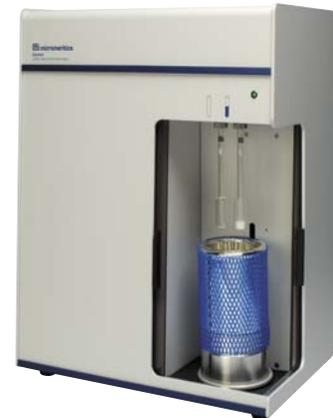
The Micromeritics Gemini V series rapidly and reliably produces accurate and repeatable surface area and porosity determinations to assure that you have reliable information about these important characteristics of your sample material. Its simplicity of use, reliability, and ruggedness has earned the Gemini its place in laboratories worldwide as an essential tool in both research and quality control environments.
