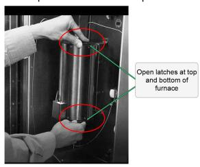
3. Open the furnace and gently pull the sample column clear of the furnace.
