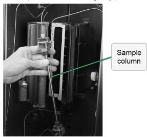
4. Place a 7/8 in. wrench on the bottom of the top sample block and a 1/2 in. wrench on the sample column nut. Loosen the nut just enough so it can be turned by hand. Repeat the process for the bottom nut.
