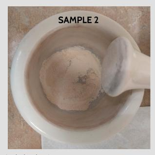
Figure 3. (left) Sample 1 - Pelletized Zeolite 13X (right) Sample 2 - Crushed Zeolite 13X
