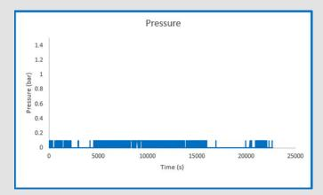
Figure 4. (left) Breakthrough adsorption curves for Pelletized Zeolite 13X (right) System pressure throughout the breakthrough experiment
