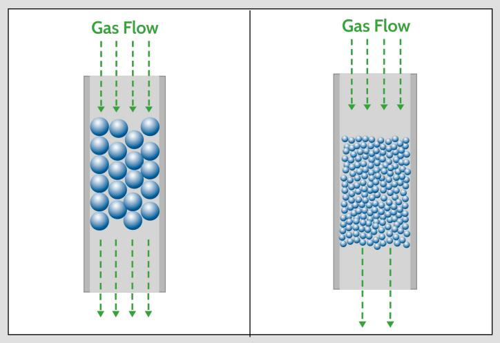
Figure 1. Illustration of particle size and pressure drop across a breakthrough column. Left) Large particles with ample interstitial space for gas to flow. Right) Small particles leaving less interstitial space leading to pressure drop across the breakthrough column.
