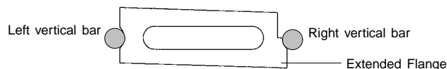
Top View of Sample Cell Seated Against Left and Right Vertical Bars
