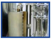
Up to 2 Extra **liquid evaporators temperature controlled** (50 to 450 °C) for heavier products or higher flow rates.
