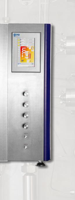
The new BreakThrough Analyzer (BTA) is a flexible gas delivery and management system for the **precise characterization** of adsorbent performance under process relevant conditions. It delivers reliable adsorption data for gas/vapor mixtures using a **flow-through system**.
