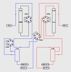
One reactor in bypass while other is in flow
