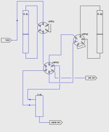
Both reactors in series with final liquid / gas separation
