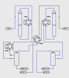
Both reactors in series and L/G Sep bypassed
