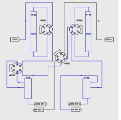
Both reactors in parallel and L/G Sep 1 in bypass
