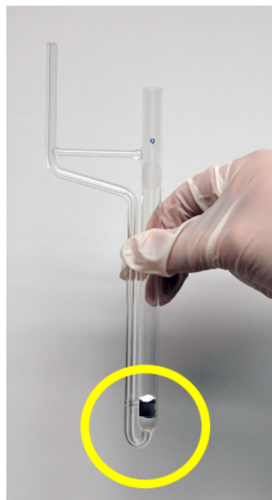
Top disc, powdered sample, bottom disc, quartz wool
