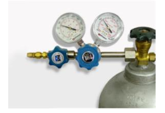
If purchased from a source other than Micromeritics, please keep in mind that many commercially available gas regulators lack key features which are required for gas adsorption measurements. These vital criteria must be met:
