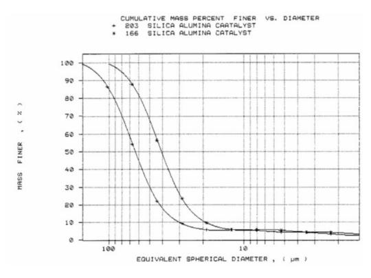
Figure 2. SediGraph PSD for Si/Al catalyst powder using (+) a sedimentation density of 1.65 g/cm3 and (\*) using a sedimentation density of 2.60 g/cm3.
