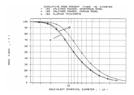
Figure 4. SediGraph PSDs (o) the precursor ATH, (+) the calcined powder, nonporous model, and (\*) the calcined powder, porous model.
